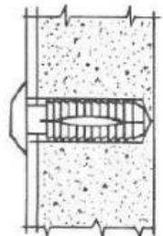
**Note:** If pin in rivet does not drive flush when fastening into solid materials and applications where expansion may be restricted, larger hole is required, use .261" - G bit.
