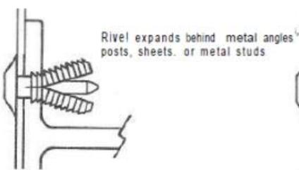
Rivet expands behind metal angles, posts, sheets, or metal studs
