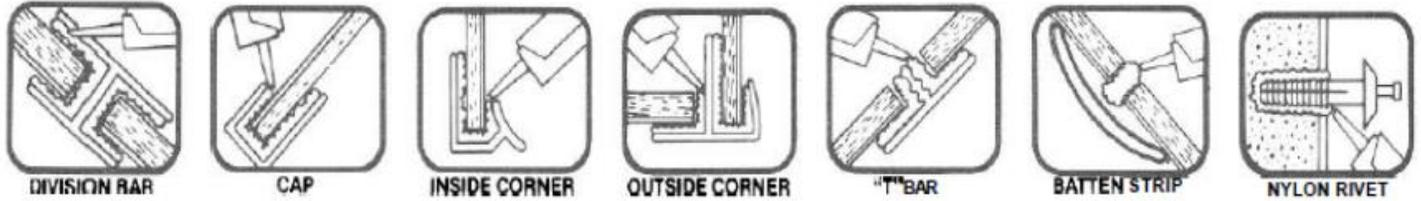
**Fasteners:** All panels should be installed with non-corroding fasteners. Plastic pin rivets, chrome pin rivets, one-piece nylon rivets, stainless nails, one stepper fasteners, or screws are recommended. See below. Fasteners should be installed to fit snug but should not be over-tightened. Always select proper fasteners for installation. Plastic pin rivet fastens panel to wood, metal, drywall, concrete, insulation materials, etc. See diagram below:
