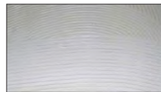
Example of properly troweled adhesive application
