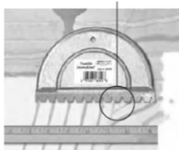
Example of properly troweled adhesive application
